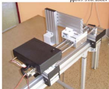
Fig 1 – Ultrasonic probe linear movement system
