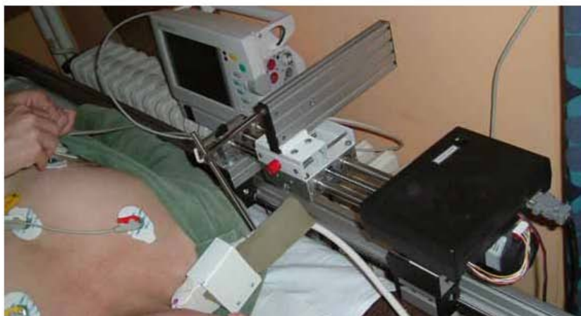
Fig. 2 Ultrasonic probe linear movement system
