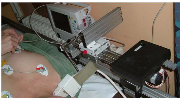
Fig. 1. Ultrasonic probe linear movement system
