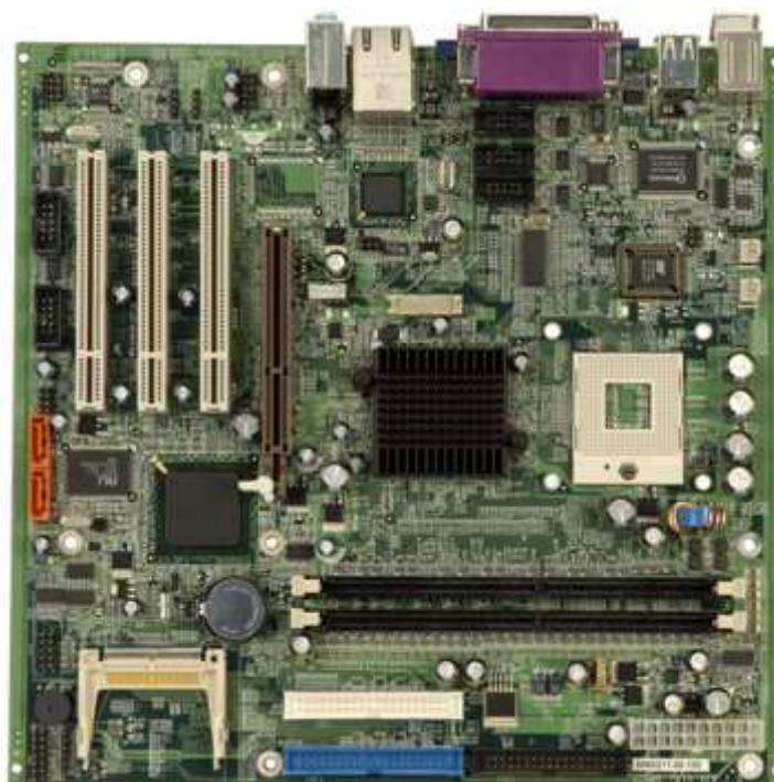
Obr. 2.26 Micro ATX SBC typu IMB-8550 s rozměry 244mm x 244mm. ( http://www.icpamerica.com/products/single_board_computers/motherboard/micro_atx/imb_8550.html )
